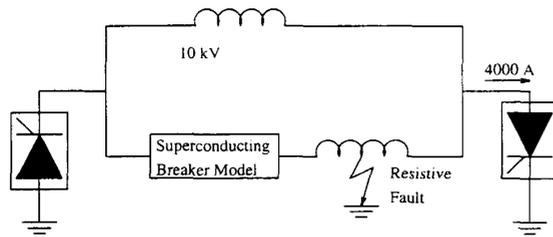
Fig. 4. Sample system for superconducting breaker example.
