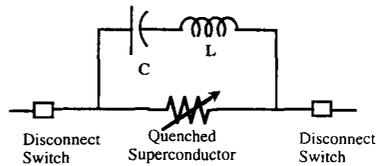
Fig. 2. Superconducting circuit breaker with LC tank to initiate current zero.
