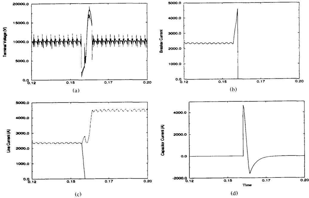
Fig. 5. Superconducting breaker during dc fault.
