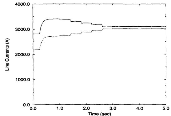
Fig. 8. Using current steering to balance line currents.
