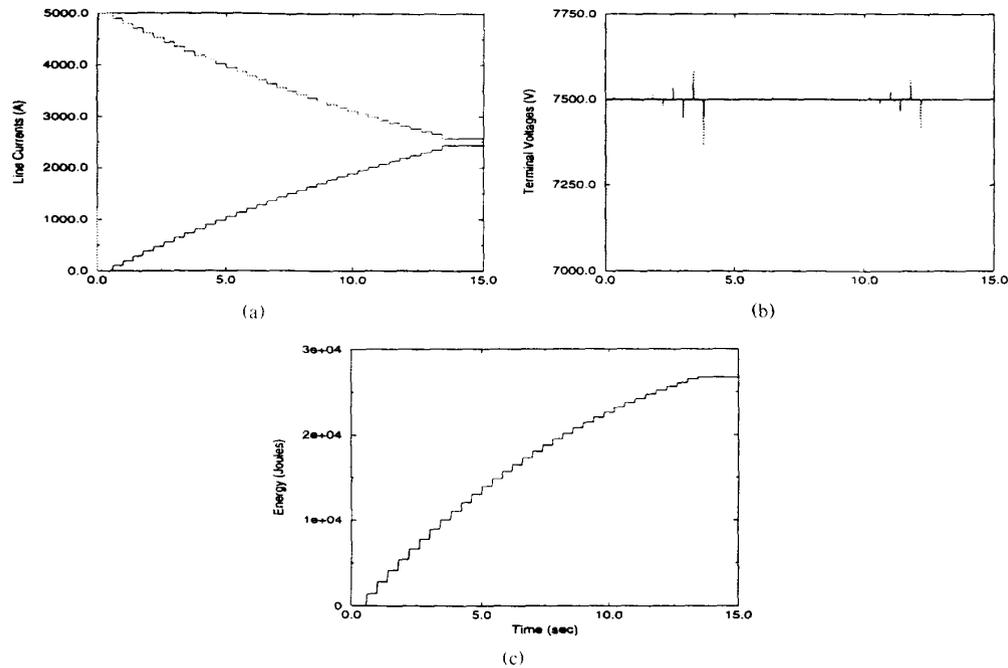
Fig. 7. Current steering to restore current in line *a* after reinsertion. (a) Currents in line *b* (top), and *a* (bottom). (b) dc voltage at rectifier 1. (c) Energy dissipated in line between rectifier 2 and inverter 5.
