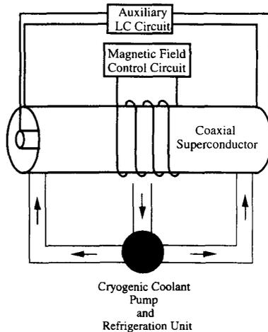
Fig. 3. Superconducting current diverter.
