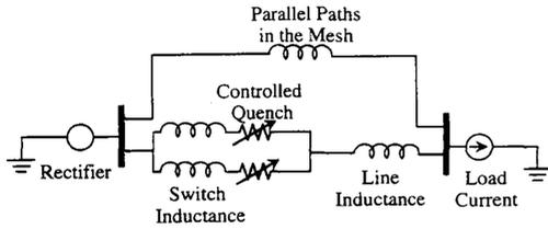
Fig. 6. Superconducting current transfer device with parallel legs.
