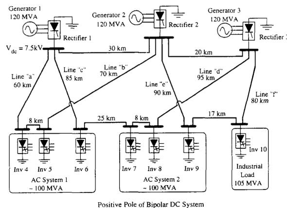
Fig. 1. Ten bus LVdc test system.
