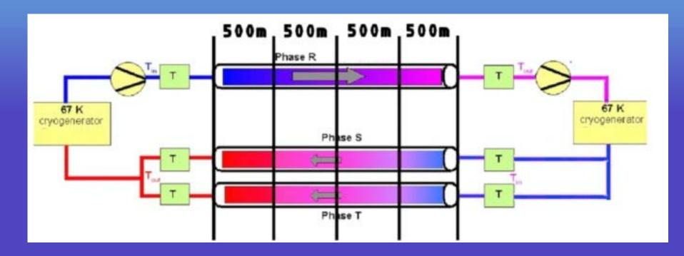
Flow of LN<sub>2</sub> in single phase and back in two phases with 2 refrigeration and pump stations
