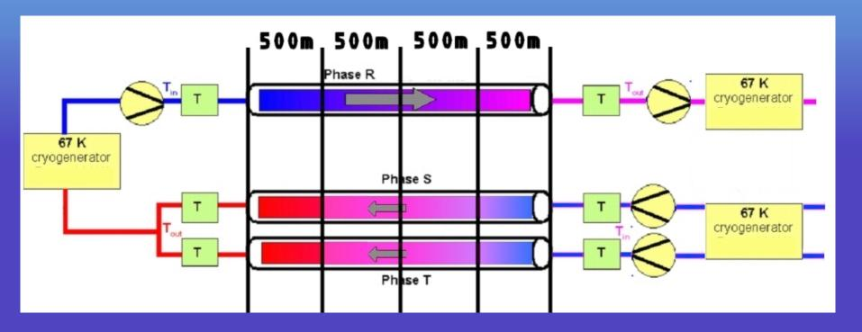
Flow of LN<sub>2</sub> in single phase and back in two phases with several refrigeration and pump stations
