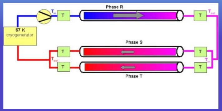
Flow of LN<sub>2</sub> in single phase and back in two phases
