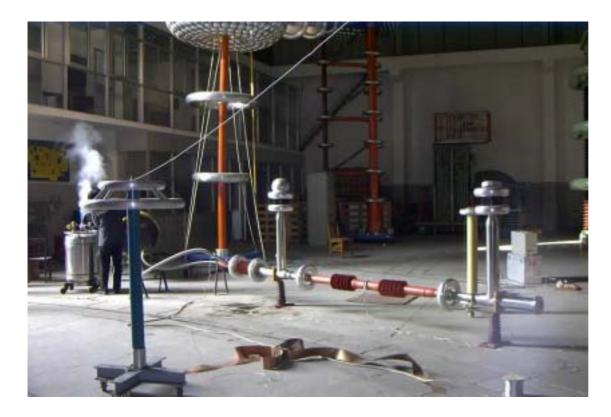
Factory sample test: Partial discharge(ac 39kV) <10 pc AC withstand voltage 65 kV, 4h, passed Joule heat at 1220A at working: 52 W Heat inleak: 38-42 W
