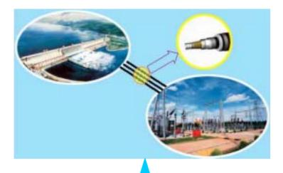
From generator to transformer, typically, 24kV/20-30kA, 20-200m
