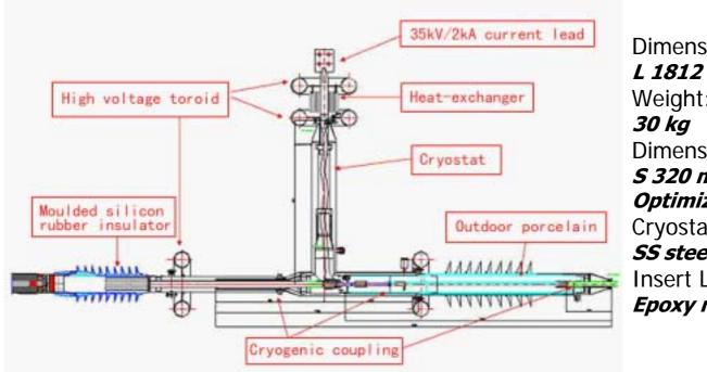
Dimension: *L 1812 mm; H 1468 mm* Weight: *30 kg* Dimension of current lead: *S 320 mm<sup>2</sup>; L 860 mm Optimized at 1220 A* Cryostat: *SS steel, evacuated* Insert LN2 pipe: *Epoxy resin tube*
