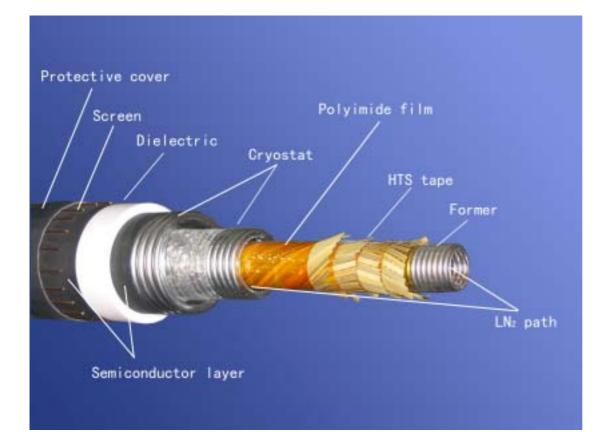
Former ID/OD(with Braiding): *30/35 mm* Layers of HTS tape: 4 Number of HTS tape: 90(21,24,24,21) Ic of HTS tape: 60-80 A (77K, self field) ID/OD of cryostat: 43/70 mm **Dielectric material:** XLPE Thickness of dielectric: 11.9mm Overall linear specific weight: 9.2kg/m
