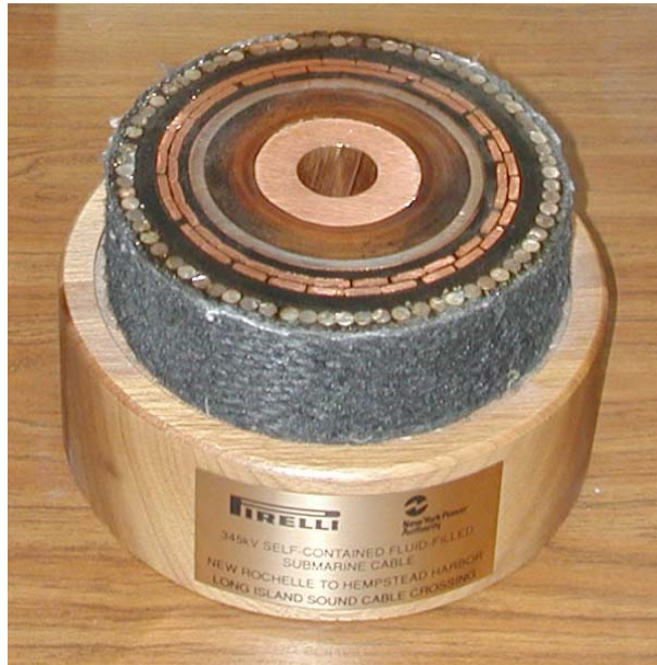
Figure III.12.1 One Phase of a 345 kV, Self-Contained Fluid (Oil) Filled Cable The cooling fluid (oil) resides in the central channel within the copper conductor.
