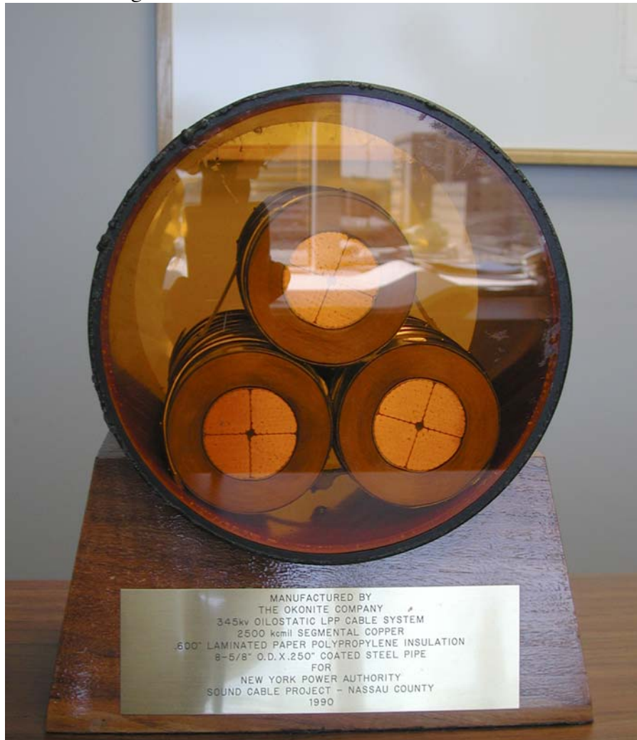
Figure III.12.2 345 kV, 760 MW Cable of the High Pressure Fluid (Oil) Filled Pipe Design
