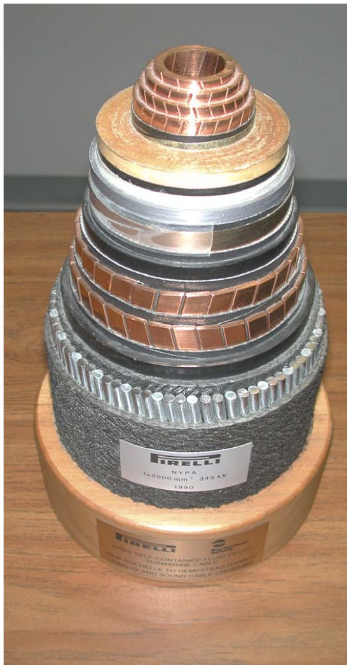
Figure X.5.2 One of the Four 345 kV Submarine AC Cables of the Self Contained Fluid (Oil) Filled Pipe Design Under Long Island Sound
