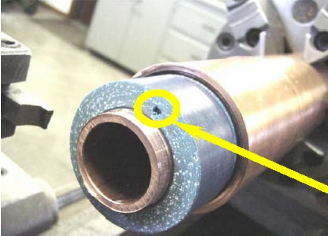
Figure VI.6.1 Undesirable Void Within Solid Dielectric
