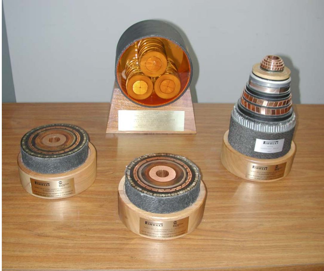
Figure X.5.1 Three Cross-Sections 345 kV Submarine AC cables of the Self Contained Fluid (Oil) Filled Pipe Design Under Long Island Sound and the Three Phase HPFF Underground Cable to which Submarine Cables Connect
