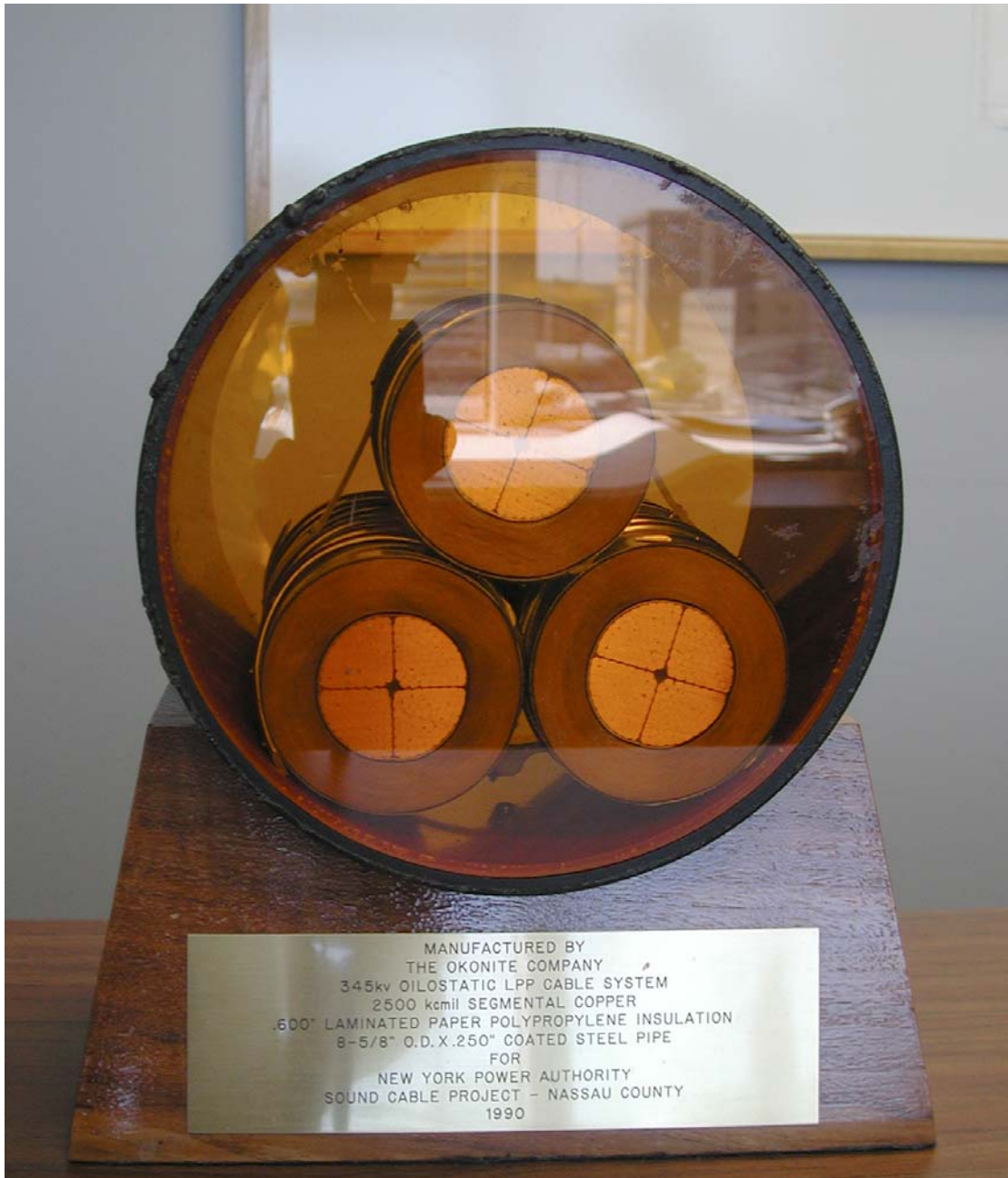
Figure X.4.2 345 kV, 760 MW Cable of the High Pressure Fluid (Oil) Filled Pipe Design
