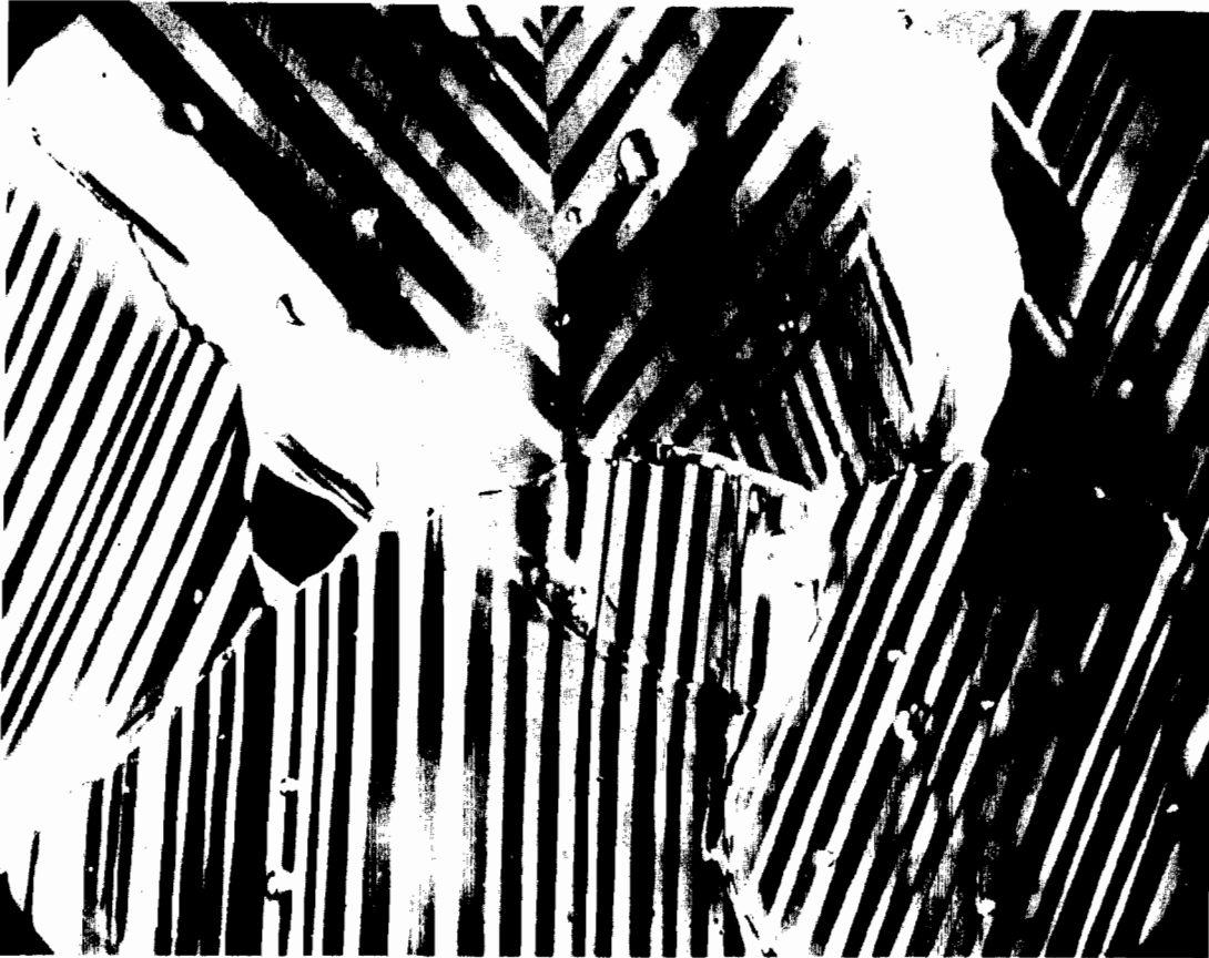
Figure 54 "Nomarski" interference contrast micrograph of In 20.9 At% Tl polycrystal, showing primary transformation lamellae. 200X
