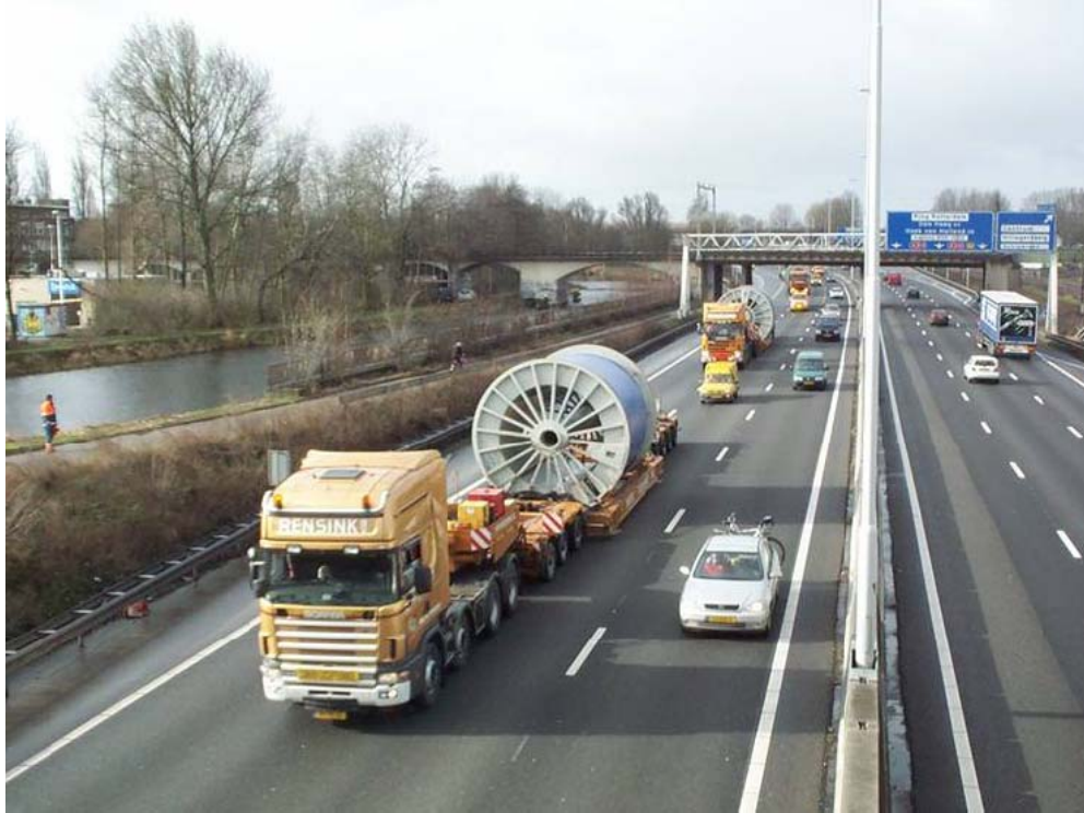
Figure 4-2 Loaded cable transport drums being transported from manufacturing facility to installation site
