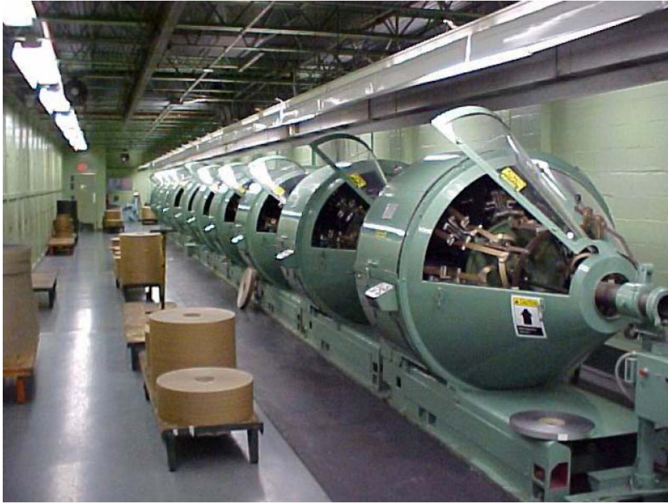
Figure 4-4 A tape-lapping machine in a humidity-controlled enclosure
