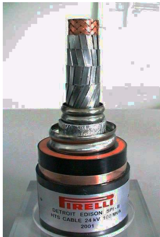
Figure 4-9 A warm dielectric, single-phase superconducting ac cable
