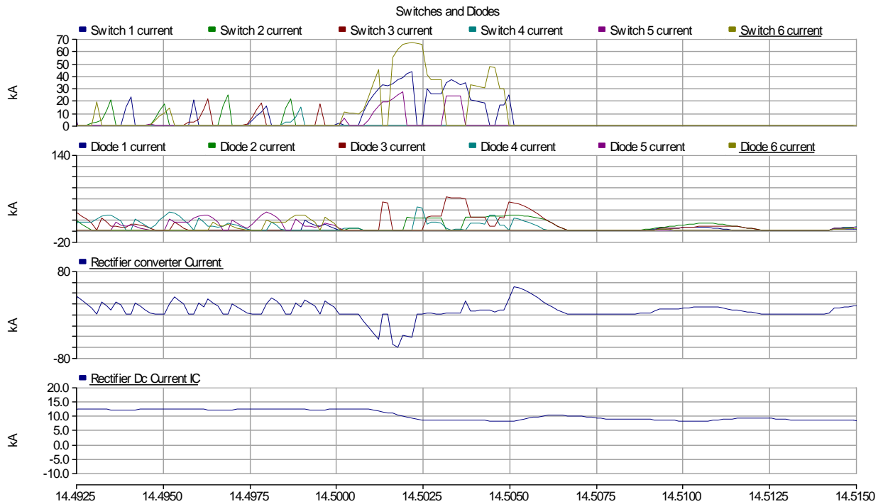
Figure 3-35 Sending end converter currents prior to and just after the application of the three phase bus fault
