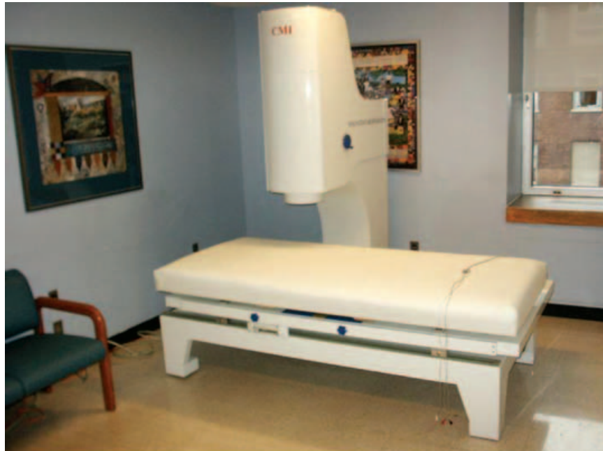
Figure 1. The CMI magnetocardiograph is a SQUID-based device operating without the need of magnetically shielded rooms. An array of nine channels senses the heart magnetic field, three additional channels are used for referencing, and one channel for reference ECG. MCG data are acquired at 36 locations above the torso by making four sequential measurements. In each position, the nine sensors measure the cardiac magnetic field for 90 seconds using a sampling rate of 1000 Hz leading to 36 individual time series. The operation of the system is computer-controlled and largely automated. The acquired signals are processed by proprietary medical application software capable of filtering, averaging, electric/magnetic activity localization, heart current reconstruction, and derivation of diagnostic scores. The device is has just recently been approved by the FDA.
