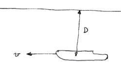
We replace, on hydrody. principle, the object with a fluid source. Contine: x-utFor invaside fluid  $\nabla^2 q = 0$ , instational, qexists:  $\vec{\tau} = \operatorname{grad} q$ .
