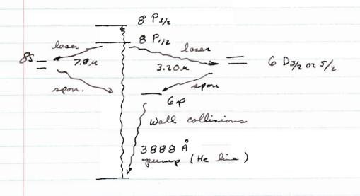
This has been the only optically pumped gas laser.
