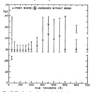
Fig. 18. Wavelength region where  $|\partial n/\partial R| \ge 20$  as a function of film thickness. The optical constants of Ge from Ref. 9 were used in Ref. 15 to calculate this bar diagram. The criterion on  $|\partial n/\partial R|$  was determined by stipulating that an error of 0.5 absolute in the derived n would be considered intolerable for an error of 2.5% absolute in the measured R.
