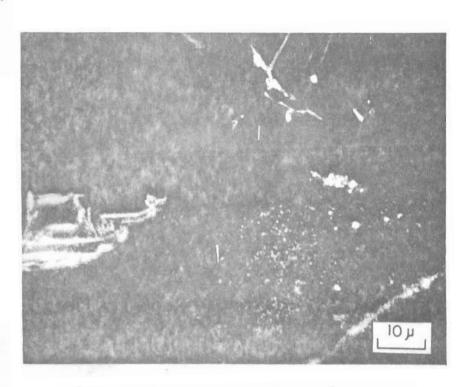
FIG. 2-7 SURFACE PHOTOMICROGRAPH OF EPITAXIAL Ge FILM ON CLEAVED CoF2
