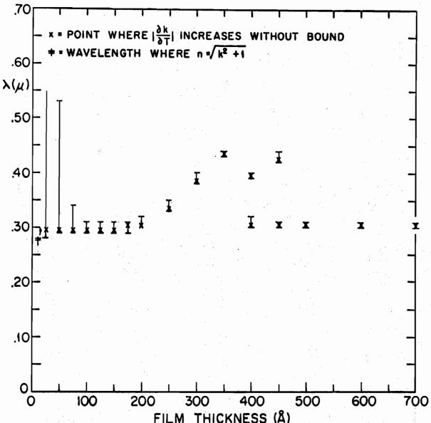
FILM THICKNESS (Å) FIG. 3-156 WAVELENGTH REGION WHERE TI  $\frac{\partial k}{\partial T}$  |  $\geq$  5 FOR THE R-T MODEL OF A Ge FILM ON CoF2.
