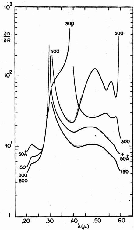
FIG. 3-110 THE INDEX OF REFRACTION ERROR DERIVATIVES VS. λ FOR THE R-T MODEL OF A Ge FILM ON Co F2.
