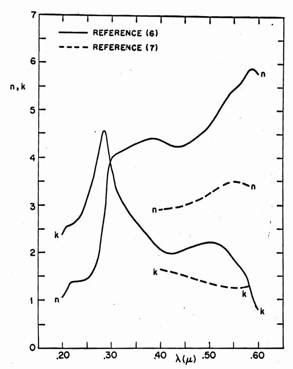
FIG. 1-5a OPTICAL CONSTANTS OBTAINED BY OTHER WORKERS FROM GERMANIUM THIN FILMS.
