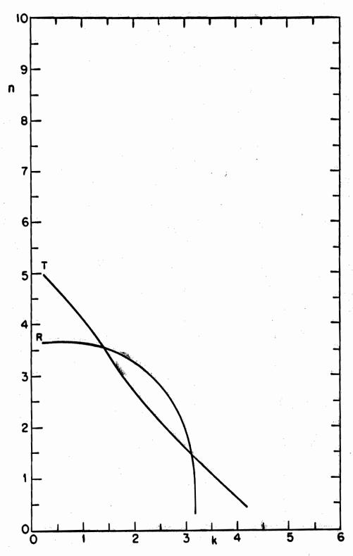
FIG. 3-60 THE ROOT-LOCUS DIAGRAM FOR THE R-T MODEL OF A 50Å Ge FILM ON COF2.  $\lambda$  = 2500Å.
