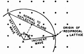
FIG. 2-5 EWALD'S CONSTRUCTION IN THE RECIPROCAL LATTICE
