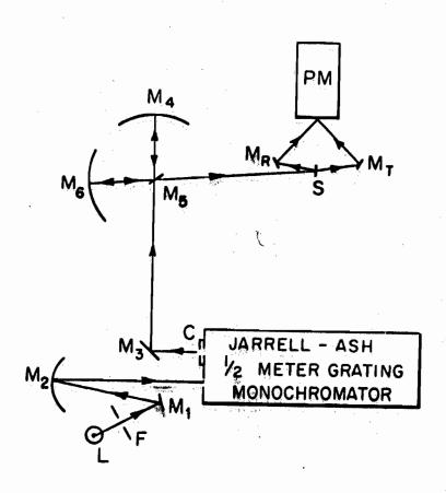
FIG. 4-10 SCHEMATIC DIAGRAM OF THE OPTICAL SIGNAL PATH.
