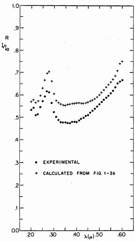
FIG. 4-120 REFLECTIVITY OF A 250Å EPITAXIAL GERMANIUM FILM ON CoF2.
