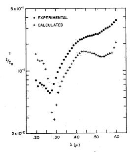
Fig. 15. Transmissivity of the same 135-Å film as in Fig. 14 compared to theoretical values calculated from the data of Ref. 9.
