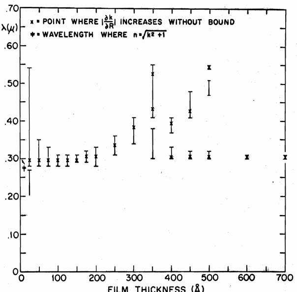
FILM THICKNESS (Å) FIG 3-150 WAVELENGTH REGION WHERE  $|\frac{\partial k}{\partial R}| \ge 20$  FOR THE R-T MODEL OF A Ge FILM ON CoF2.
