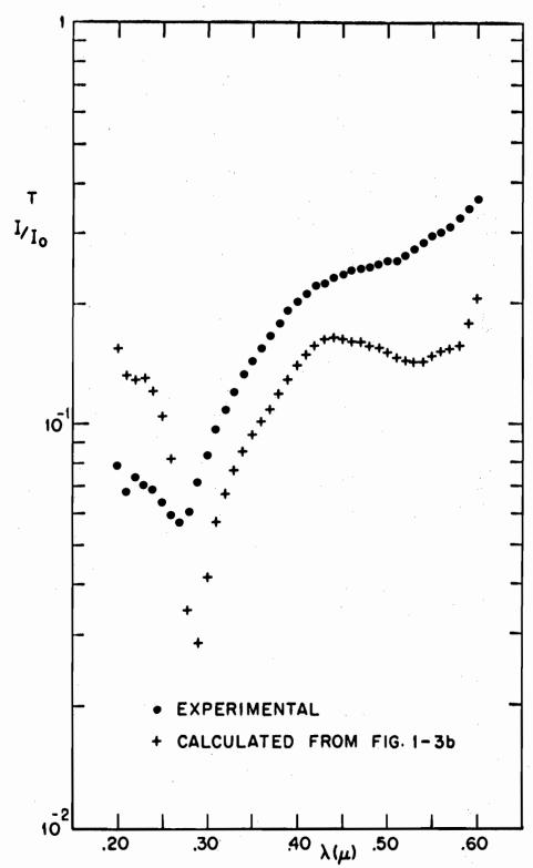
FIG. 4-136 TRANSMISSION OF A 135Å EPITAXIAL GERMANIUM FILM ON CoF2.
