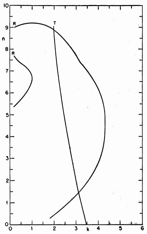
FIG. 3-80 THE ROOT-LOCUS DIAGRAM FOR THE R-T MODEL OF A 300 Å Ge FILM ON GOF2.  $\lambda$  2500Å.
