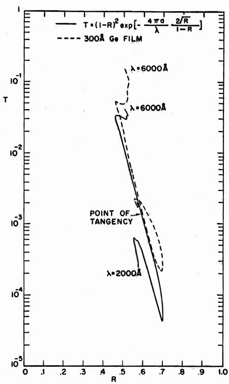
FIG. 3-5 A T VS. R REPRESENTATION USING RELATION (3-12) AND R AND T FOR A 300Å Ge FILM CALCULATED FROM EQUATIONS (3-90) AND (3-10).
