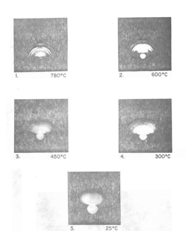
FIG. 4-6 RED PATTERNS FOR Ge FILMS ON FUZED QUARTZ FOR VARIOUS SUBSTRATE TEMPERATURES, Ts. Δ APPROXIMATELY CONSTANT.
