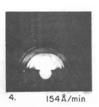
FIG. 4-8 RED PATTERNS FOR Ge FILMS ON FUZED QUARTZ FOR VARIOUS DEPOSITION RATES, Δ. Ts = 600°C.
