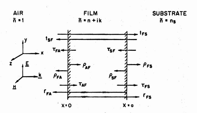
FIG. 3-1 MODEL FOR THE CASE OF AN ABSORBING THIN FILM ON A SEMI-INFINITE NON-ABSORBING SUBSTRATE.
