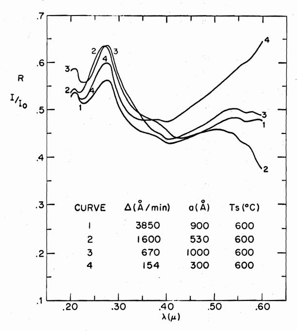
FIG. 4-9. REFLECTIVITY OF Ge FILMS ON FUZED QUARTZ FOR VARIOUS DEPOSITION RATES, Δ.
