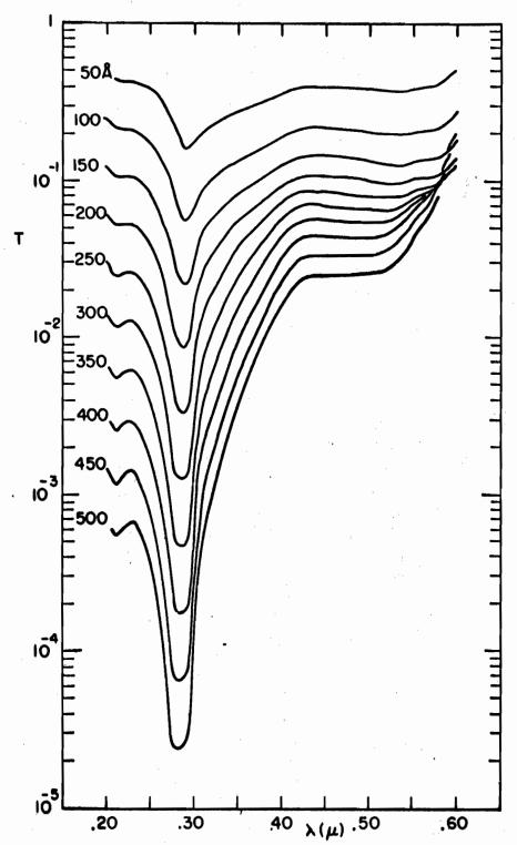
FIG. 3-3 THE TRANSMISSION OF GERMANIUM THIN FILMS ON CoF2 SUBSTRATES USING THE OPTICAL CONSTANTS DERIVED BY PHILIPP(2). THE FILM THICKNESS IS INDICATED FOR EACH CURVE.
