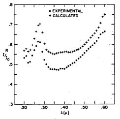
Fig. 12. Reflectivity of a 250-Å epitaxial film on CaF<sub>2</sub> compared to theoretical values calculated from the data of Ref. 9.
