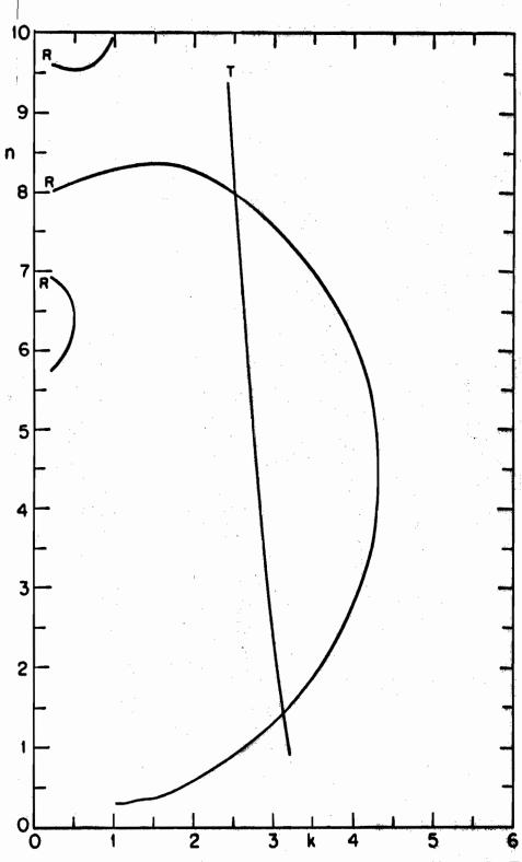
FIG. 3-90 THE ROOT-LOCUS DIAGRAM FOR THE R-T MODEL OF A 500Å Ge FILM ON COF2.  $\lambda$  = 2500Å.
