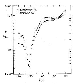
Fig. 13. Transmissivity of the same 250-Å film as in Fig. 12 compared to theoretical values calculated from the data of Ref. 9.
