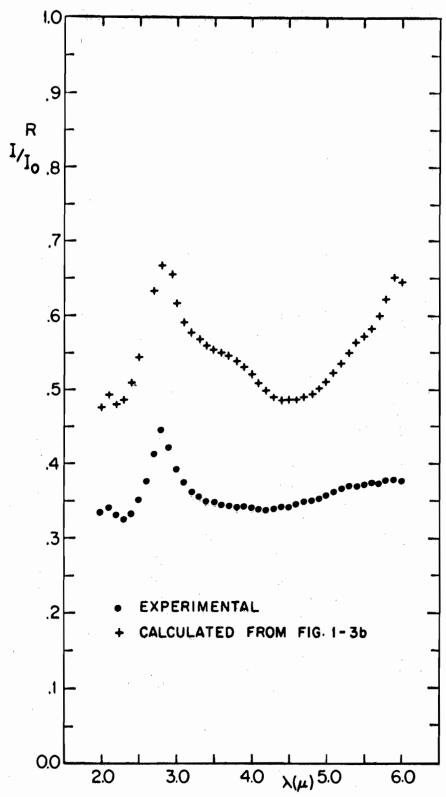
FIG. 4-130 REFLECTIVITY OF A 135Å EPITAXIAL GERMANIUM FILM ON CoF2.
