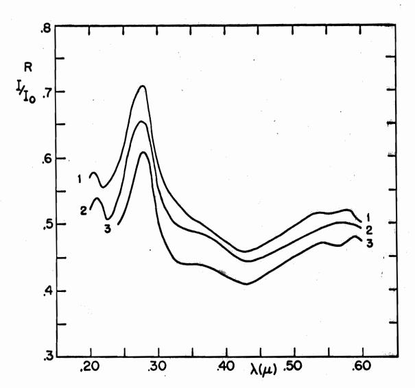
FIG. 1-30 REFLECTIVITY OF BULK GERMANIUM.
