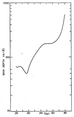
Fig. 4. Skin depth of germanium as a function of wavelength.
