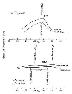
Fig. 17. Effect of film stress on the reflectivity peaks of the 1850-Å epitaxial Ge film on CaF<sub>2</sub>.
