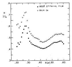
Fig. 11. Reflectivity of a 1850- $\mathring{\rm A}$  epitaxial germanium film on CaF<sub>2</sub> compared to that of bulk germanium.
