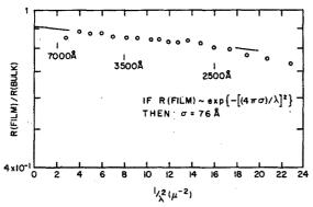
Fig. 16. Plot of R(film)/R(bulk) vs  $1/\lambda^2$  for the 1850-Å epitaxial Ge film on CaF<sub>2</sub>.
