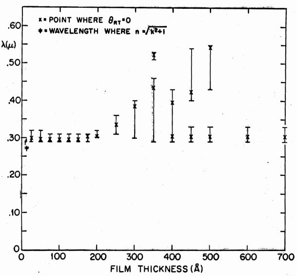
FIG. 3-13 WAVELENGTH REGION WHERE 101<sub>RT</sub> ≤10° FOR THE R-T MODEL OF A Ge FILM ON CoF2.
