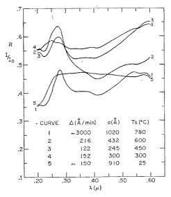
Fig. 9. Reflectivity of Ge films on fused quartz for various substrate temperatures.  $\Delta =$  deposition rate, a = film thickness,  $T_8 =$  substrate temperature.
