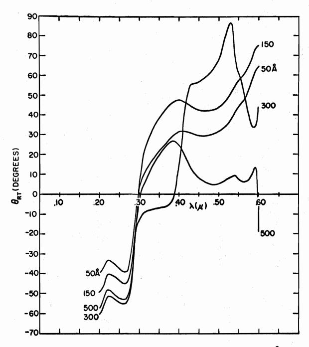
FIG. 3-10 THE ANGLE OF ROOT-LOCUS INTERSECTIONS,  $\theta_{RT}$ , VS.  $\lambda$  FOR THE R-T MODEL OF A Ge FILM ON CGF2. FILM THICKNESS IS INDICATED ON EACH CURVE.
