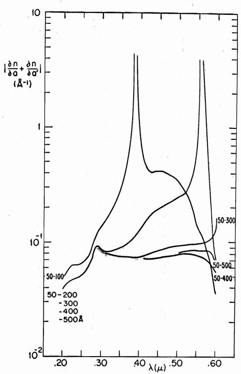
FIG. 3-17a THE INDEX OF REFRACTION COMBINED THICKNESS ERROR DERIVATIVES VS. X FOR TWO THICKNESS, TWO TRANSMISSION METHOD FOR Ge FILMS ON CaF2.
