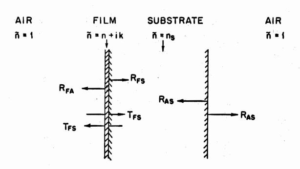
FIG. 3-2 INTENSITY ADDITION MODEL FOR A THIN ABSORBING FILM ON A THICK NON-ABSORBING SUBSTRATE.
