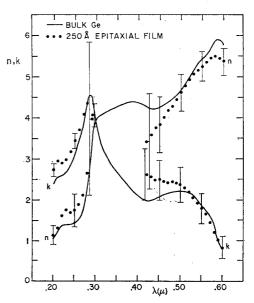
Fig. 19. Optical constants derived from R and T measurements on a 250-Å epitaxial germanium film deposited on  $CaF_2$ .
