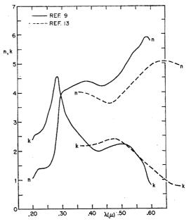
Fig. 6. Optical constants obtained by Lukes from germanium thin films, shown by the broken line. The solid line indicates Philipp's calculations from the data of Donovan et al.
