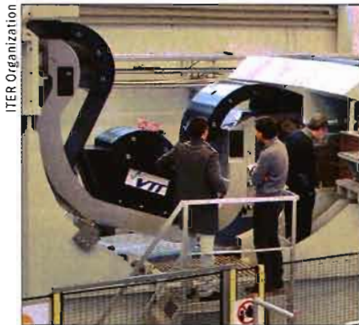
ITER Organization The ITER tokamak will use 54 divertor cassettes to funnel out waste particles and heat 9
