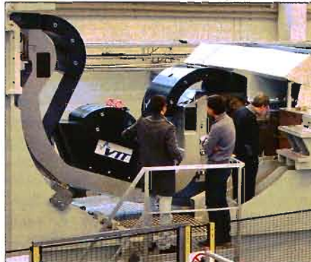
Carefully does it Researchers at the VTT Technical Research Centre in Tampere, Finland, practise inserting a dummy cassette of the type that will be used in the ITER fusion reactor, which is currently being built in France.
