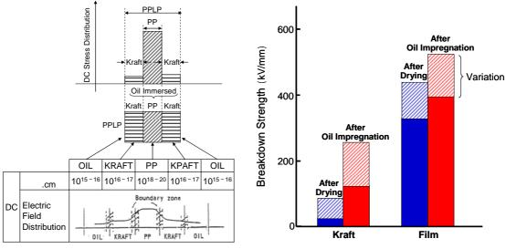
Figure 4. & Electrical Field Distribution of PPLP
