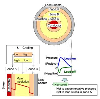
Figure 16. Countermeasures against Negative Pressure Arising at Load-off
