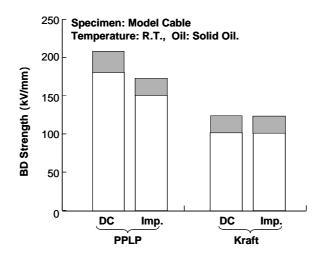
Figure 6. DC & Imp. BD Strengths of PPLP & Kraft
