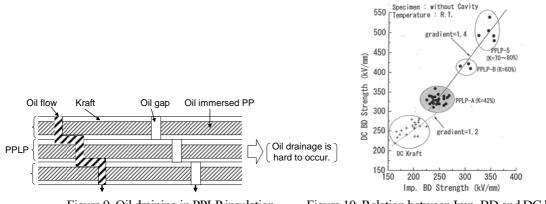
Figure 9. Oil draining in PPLP insulation
