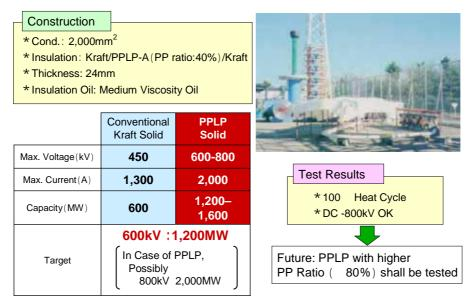
Figure 12. Test on PPLP 800kV Solid (MI) DC Cable at SEI's Kumatori Testing Station
