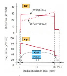
Figure 8. DC 500kV 1×3,000mm<sup>2</sup> Submarine cable with PPLP/Kraft Insulation (22.5mm)
