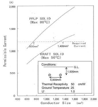
Figure 14. PPLP or Kraft Solid DC Cable of 250kV 1×1,200A Project
