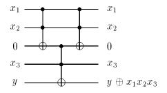
The purpose of the last  $\theta^{(3)}$  gate is to reset the scratch bit back to its original value zero. Actually, with one more gate we can obtain an implementation of  $\theta^{(4)}$  that works irrespective of the initial value of the scratch bit:
