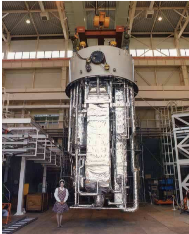
Figure 12-8 Large Liquid Helium Refrigerator (JAERI)
