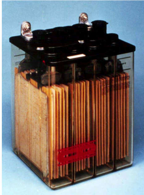
Figure 6-1 A Flooded Stationary Lead-Acid Cell (Courtesy C&D Technologies, Inc.)
