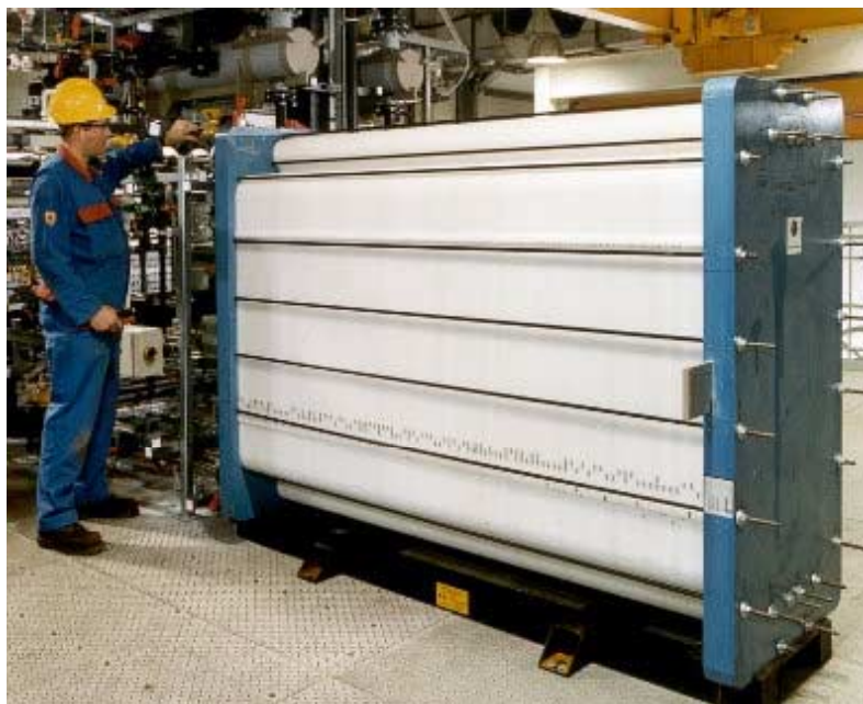
Figure 11-4 Regenesys 100 kW dc XL Module
