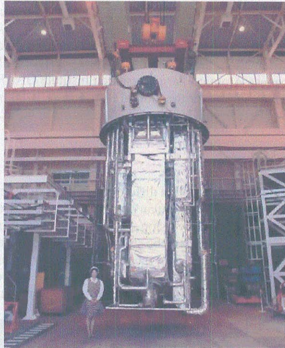
Figure 12-8 Large Liquid Helium Refrigerator (JAERI)
