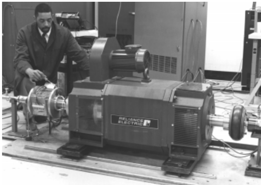
Fig. 1.2. World-record 200 hp HTS motor tested by Reliance/DOE team in early 1996.
