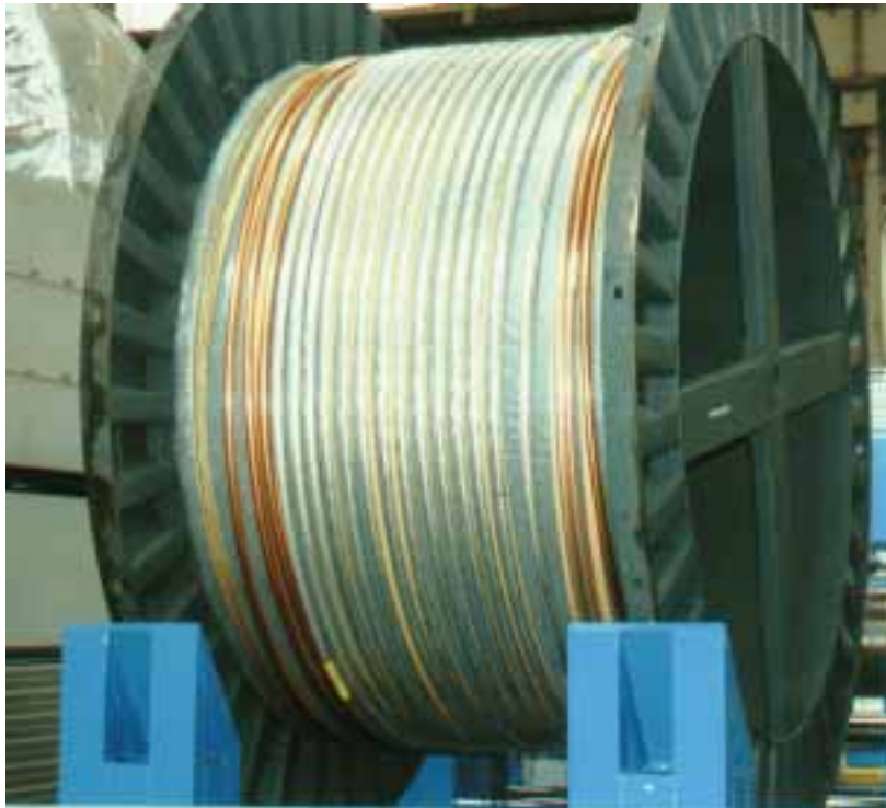
Fig. 3.3. Fifty-meter-long cabled conductor coil.
