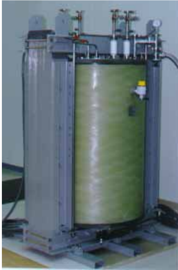
Fig. 3.6. Fuji/SEC/Kyushu University HTS transformer unit.
