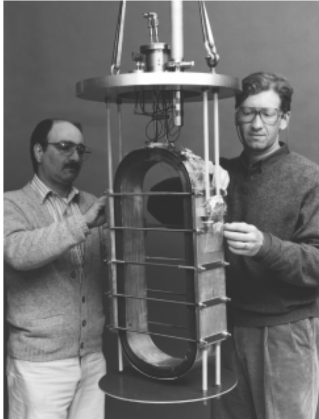
Fig. 2.4. General Electric prototype Bi-2223 racetrack coil for generator application.
