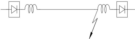
Fig. 3 Flashover of line-end bushing of inverter-side smoothing reactor
