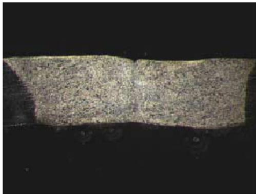
**Fig. 14. Tube 3 - crack location**
