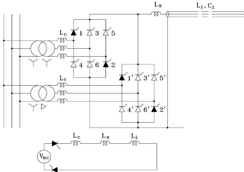
Fig. 4. Representation of a 12-pulse parallel-connected rectifier bridge with fault at inverter end.  $L_c$  = commutating inductance;  $L_s$  = smoothing inductance;  $L_l, C_l$  = inductance and capacitance of the cable.
