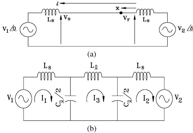
Fig. 7. Schematic representations of the dc cable system for harmonic analysis. (a) 3-GW 100-km cables; (b) 500-MW 500-m cables.  $V_1, V_2$  = harmonic voltage sources;  $L_s$  = smoothing reactors;  $L_l, C_l$  = total inductance and capacitance of cable.
