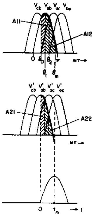
Fig. 5. Voltage across 12-pulse rectifier bridge and current profile under fault condition.
