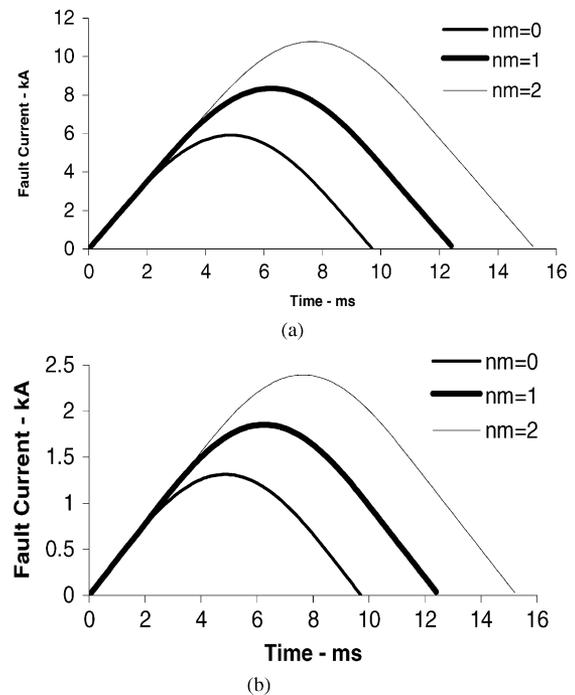
Fig. 6. Fault current profiles of the 3-GW 200-kV 100-km-long base design. Twelve-pulse converter bridge connected in parallel; commutating reactance = 0.15 p.u. (a) Smoothing reactor,  $L_s$  = 100 mH. (b) Smoothing reactor,  $L_s$  = 500 mH.
