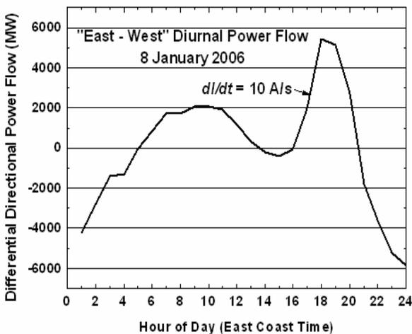
Fig. 5. East-West differential power flows as a function of EST. This plot is not intended to reflect actual magnitudes of power transfer on the SuperTie, but rather when they might occur (zero crossings) and how rapidly.
