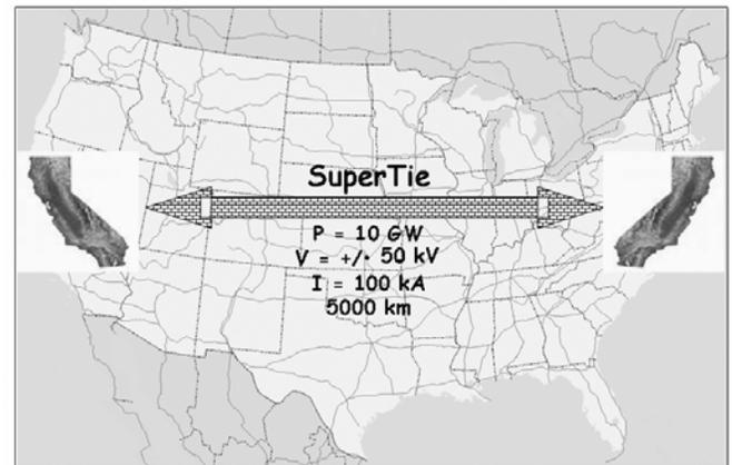
Fig. 3. Cartoon of an hypothetical continental US East-West Intertie to implement diurnal intercoastal electricity trading. For simplicity, we assume eastern electricity demand to be identical to California on any given day, shifted three hours forward relative to PST.
