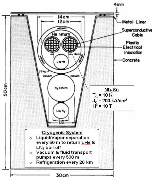
Fig. 1. Cross-sectional view of the Garwin-Matisoo 1000 km, 100 GW LHe-cooled  $\text{Nb}_3\text{Sn}$  based superconducting dc cable, taken from Fig. 1 taken from their 1967 paper [1], with annotations added by the present author.
