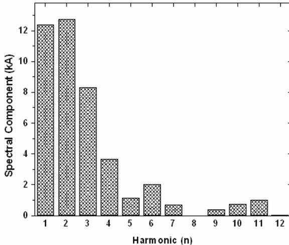
Fig. 6. Spectral distribution of the time dependence intercoastal power demand plotting in Fig. 5. The period is 24 hours, thus the first harmonic frequency is 11.6  $\mu$ Hz.
