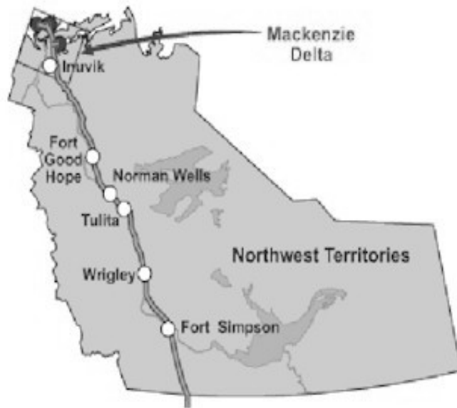
FIGURE 5. Route of the projected Mackenzie Valley Pipeline running 1220 km through the Canadian Northwest Territory from the Mackenzie River Delta on the Arctic Ocean to northern distribution channels in the province of Alberta [ http://www.mackenziegasproject.com ]. When completed, the pipeline will convey 1.6 US billion cubic feet per day, the equivalent of 18 GW thermal at the high heat value of methane, approximately that of the electric power capacity of the Three Gorges hydroelectric facility in China.
