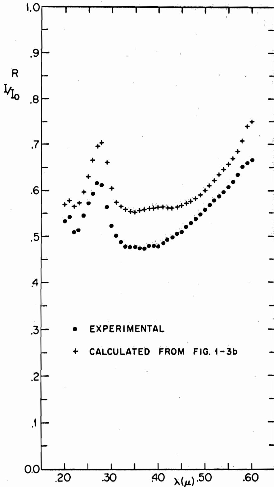
FIG. 4-12a REFLECTIVITY OF A 250Å EPITAXIAL GERMANIUM FILM ON CaF<sub>2</sub>.
