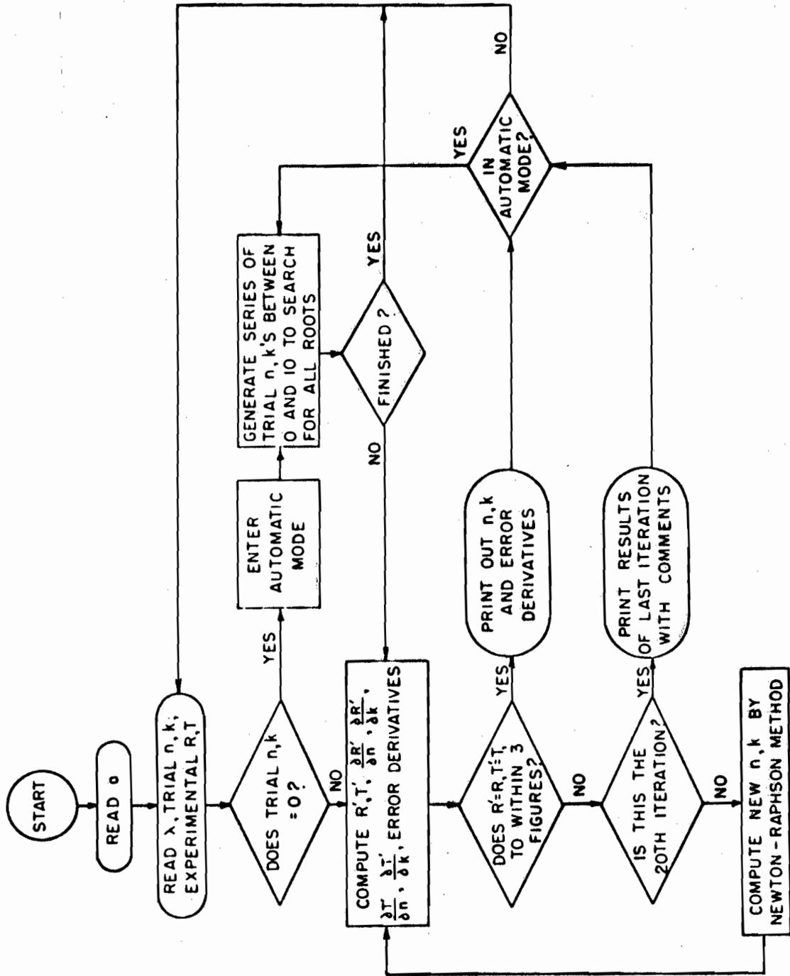
FIG 5-4 FLOW CHART OF OPTICAL CONSTANT CALCULATION PROGRAM.
