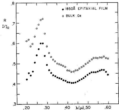
FIG. 11. Reflectivity of a 1850-Å epitaxial germanium film on CaF<sub>2</sub> compared to that of bulk germanium.
