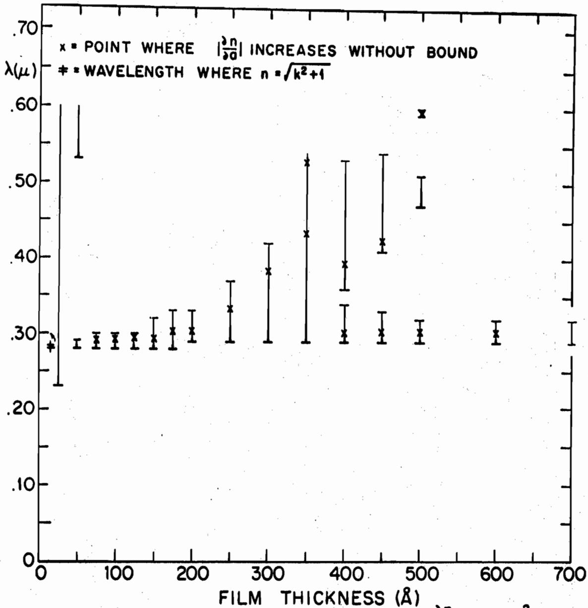
FIG. 3-14c WAVELENGTH REGION WHERE  $|\frac{\partial n}{\partial a}| > 5 \cdot 10^{-2}/\text{\AA}$
