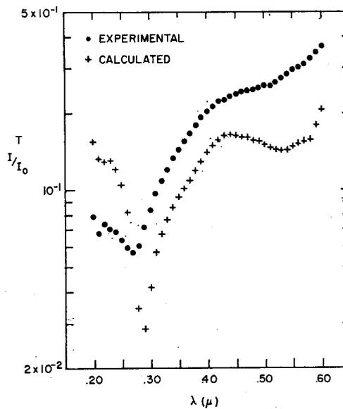
FIG. 15. Transmissivity of the same 135-Å film as in Fig. 14 compared to theoretical values calculated from the data of Ref. 9.
