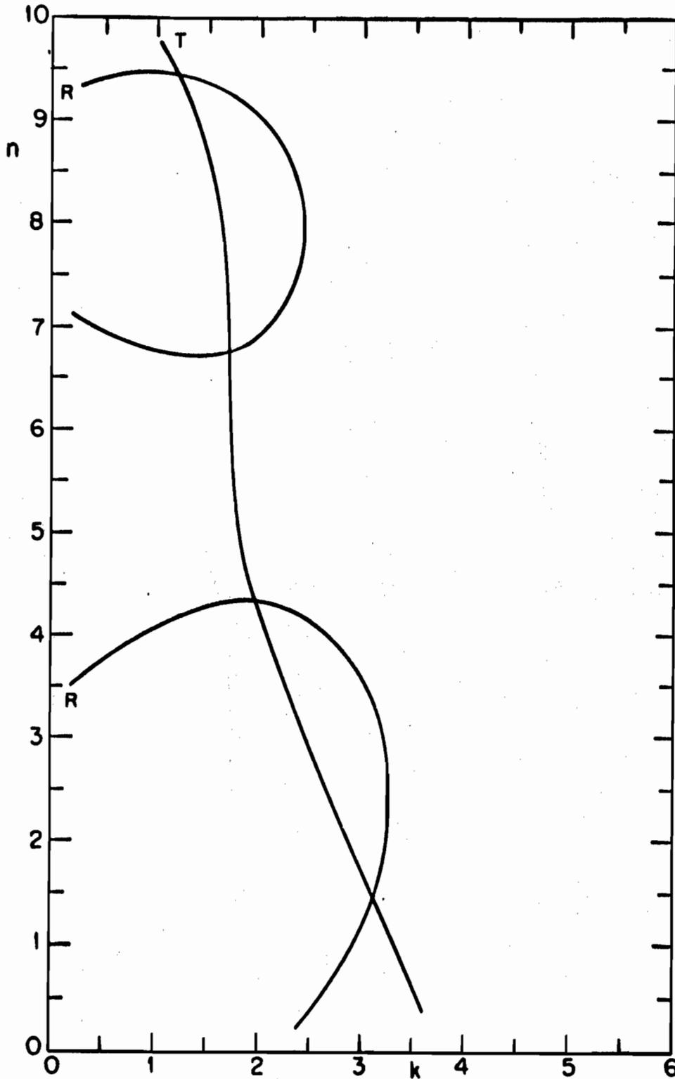
FIG. 3-70 THE ROOT-LOCUS DIAGRAM FOR THE R-T MODEL OF A 150 Å Ge FILM ON CoF<sub>2</sub>.  $\lambda = 2500 \text{ \AA}$ .
