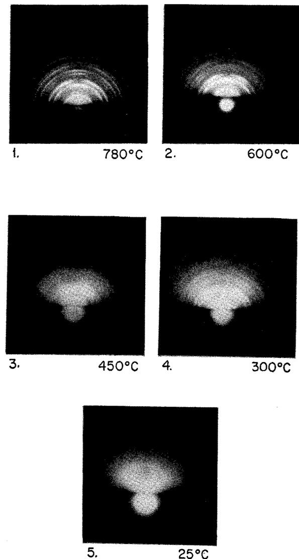
FIG. 8. Reflection electron diffraction patterns of Ge films deposited on fused quartz at various substrate temperatures. The deposition rate was from 120 to 220 Å/min for all films except film 1, where the high substrate temperature made it necessary to raise the deposition rate to 3000 Å/min in order to form a film.
