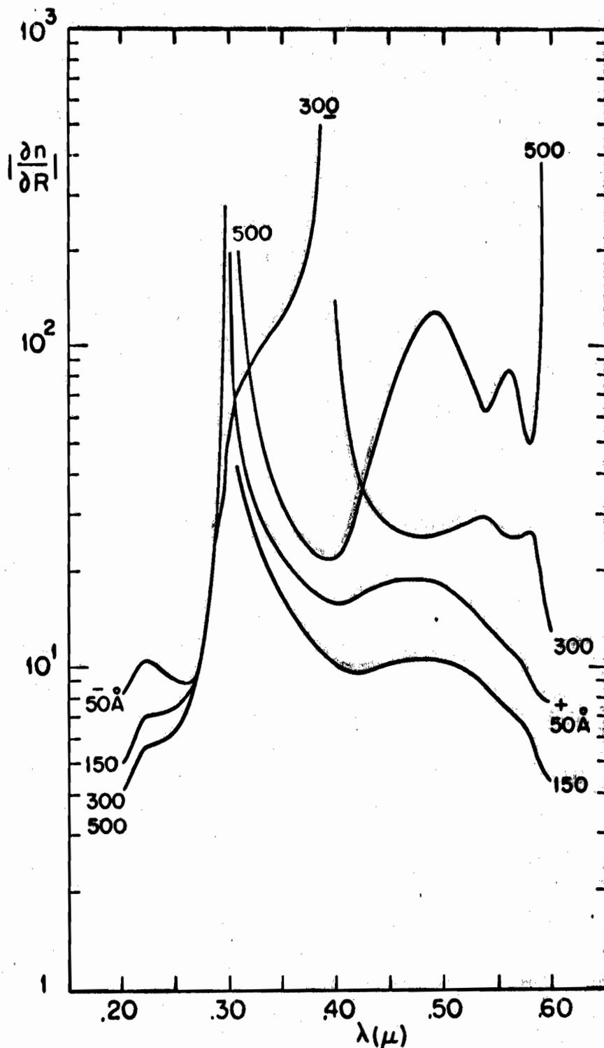
FIG. 3-110 THE INDEX OF REFRACTION ERROR DERIVATIVES VS.  $\lambda$  FOR THE R-T MODEL OF A Ge FILM ON  $\text{CoF}_2$ .
