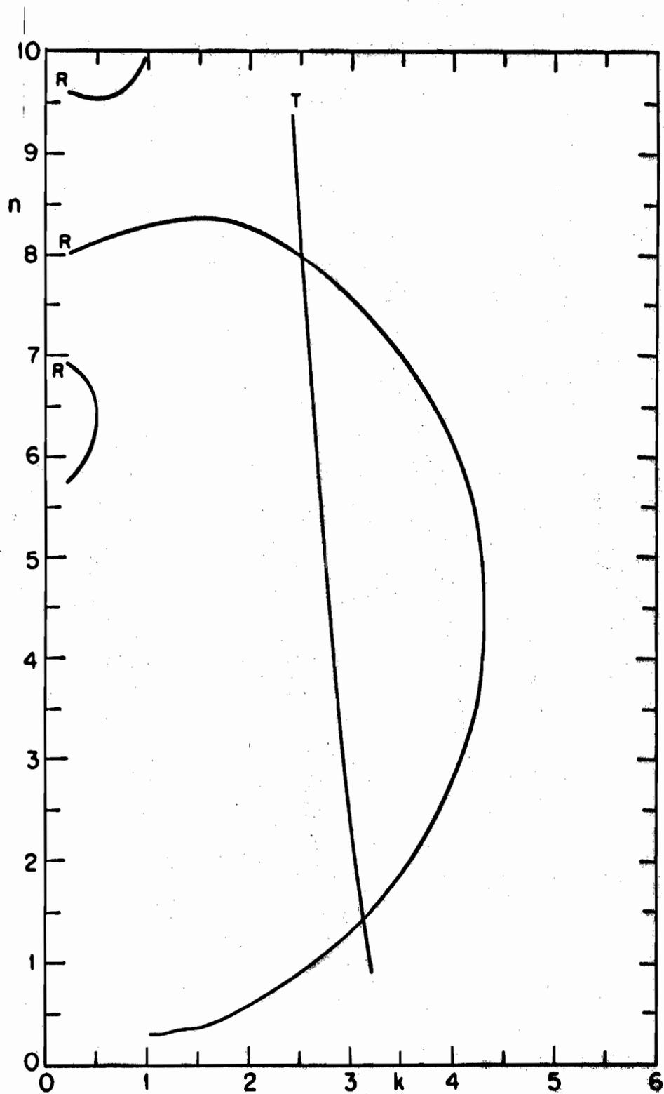
FIG. 3-9a THE ROOT-LOCUS DIAGRAM FOR THE R-T MODEL OF A 500Å Ge FILM ON CoF<sub>2</sub>.  $\lambda = 2500\text{\AA}$ .
