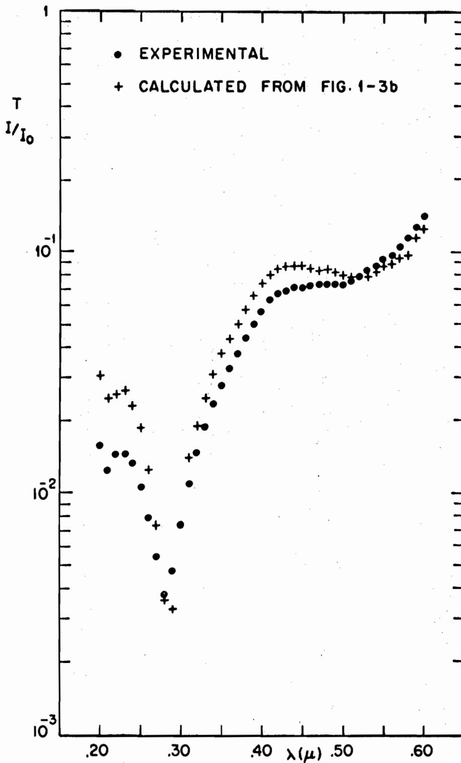
FIG. 4-12b TRANSMISSION OF A 250Å EPITAXIAL GERMANIUM FILM ON CaF<sub>2</sub>.
