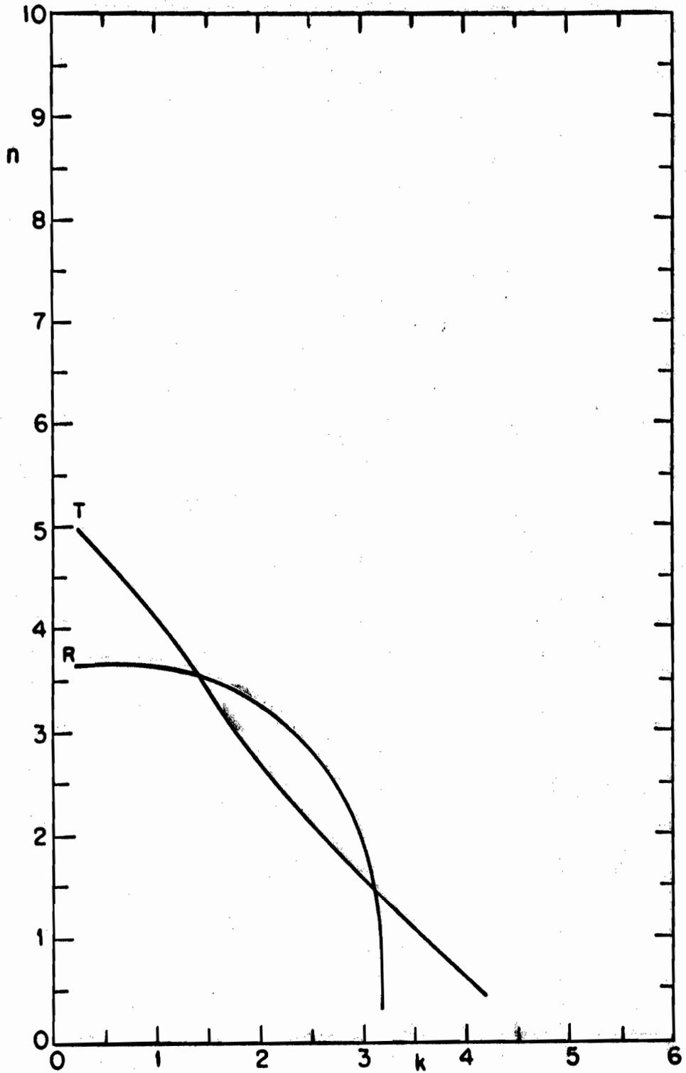
FIG. 3-6a THE ROOT-LOCUS DIAGRAM FOR THE R-T MODEL OF A 50Å Ge FILM ON CoF<sub>2</sub>.  $\lambda = 2500\text{Å}$ .
