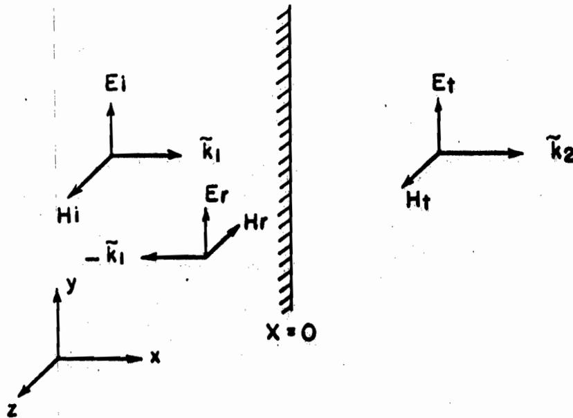
FIG. 1-1 REFLECTION AND TRANSMISSION OF AN ELECTROMAGNETIC WAVE AT THE BOUNDARY BETWEEN TWO MEDIA.
