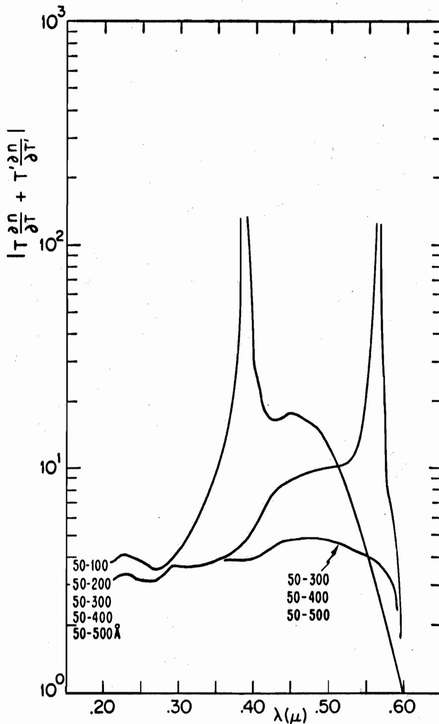
FIG. 3-16a THE INDEX OF REFRACTION COMBINED TRANSMISSION ERROR DERIVATIVES VS.  $\lambda$  FOR TWO THICKNESS, TWO TRANSMISSION METHOD FOR Ge FILMS ON  $\text{CaF}_2$ .
