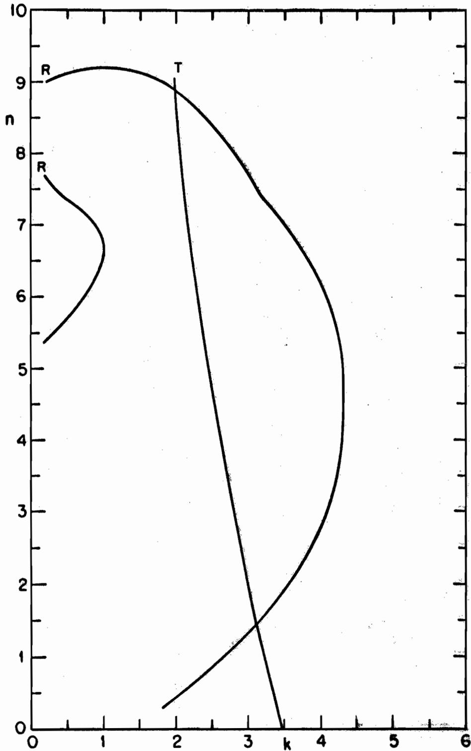
FIG. 3-80 THE ROOT-LOCUS DIAGRAM FOR THE R-T MODEL OF A 300 Å Ge FILM ON CaF<sub>2</sub>.  $\lambda = 2500\text{Å}$ .
