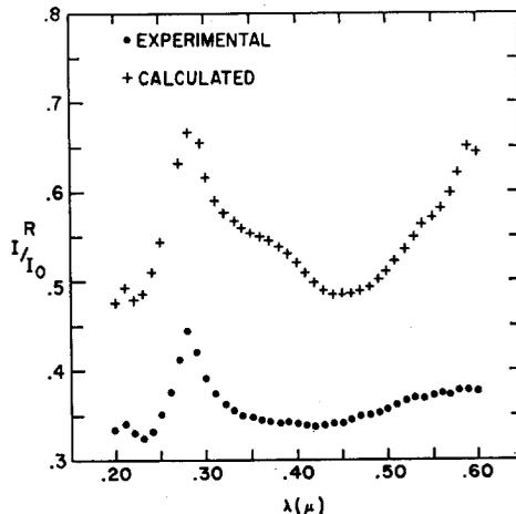
FIG. 14. Reflectivity of a 135-Å epitaxial film on CaF<sub>2</sub> compared to theoretical values calculated from the data of Ref. 9.
