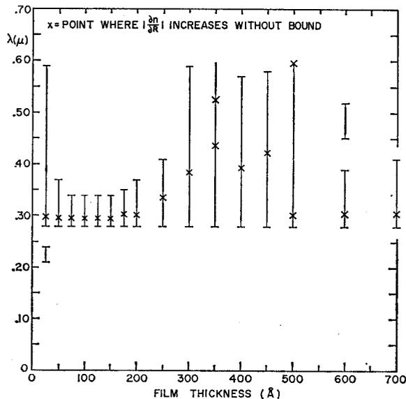
FIG. 18. Wavelength region where  $|\partial n/\partial R| \geq 20$  as a function of film thickness. The optical constants of Ge from Ref. 9 were used in Ref. 15 to calculate this bar diagram. The criterion on  $|\partial n/\partial R|$  was determined by stipulating that an error of 0.5 absolute in the derived  $n$  would be considered intolerable for an error of 2.5% absolute in the measured  $R$ .
