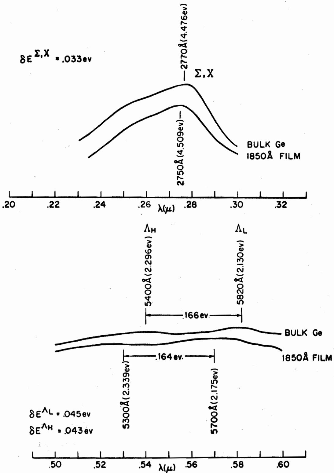
FIG. 4-15 EFFECT OF FILM STRESS ON REFLECTIVITY PEAKS.
