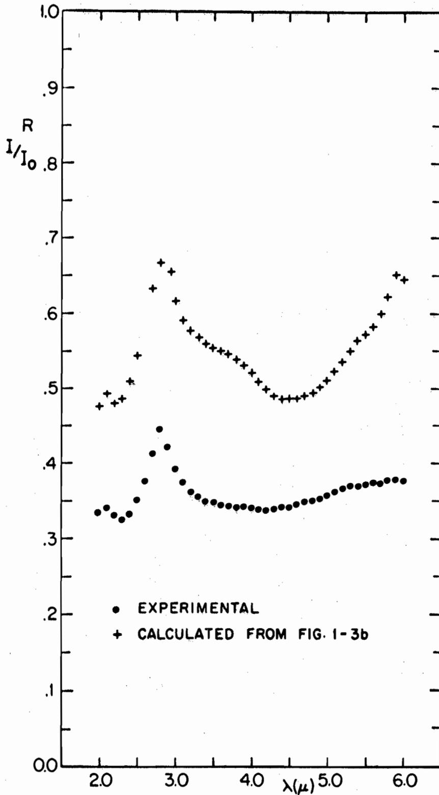
FIG. 4-13a REFLECTIVITY OF A 135Å EPITAXIAL GERMANIUM FILM ON CaF<sub>2</sub>.
