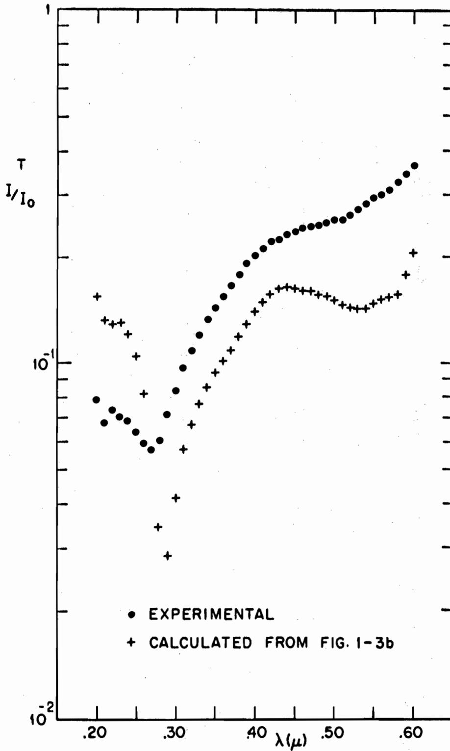
FIG. 4-13b TRANSMISSION OF A 135 Å EPITAXIAL GERMANIUM FILM ON CaF<sub>2</sub>.
