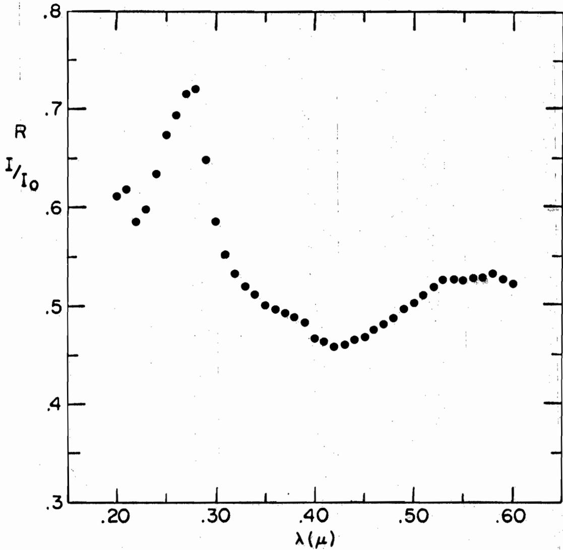
FIG. 4-5 REFLECTIVITY OF ETCHED SINGLE CRYSTAL BULK GERMANIUM.
